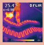
This way, the infrared waves aren't absorbed by the air but by the solid masses that transform them into thermal energy. This energy is transferred into the room, thus creating optimal conditions of comfort
